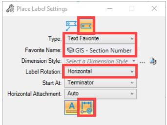
9. **Left Click** on the element to be annotated. Move the cursor where the label is to be located then **Left Click** to place the label.
